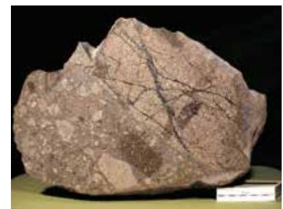
Cut surface of igneous breccia from the Flammefjeld complex. The large granitic fragmentation with stockwork molybdenum mineralisation runs 0.45% MoS 2 .
